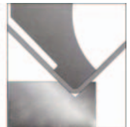
Figure 3 90° punch 1.5mm tip radius
