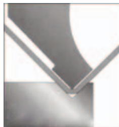
Figure 1 90° punch 0.2mm tip radius
