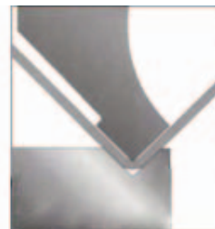
Figure 2 90° punch 0.8mm tip radius
